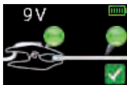
Grounding clamp detected, Coating without defect
