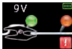
Grounding clamp detected, Coating with defect
